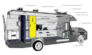
mobile solution for CBRN threats. The vehicle may include an open vehicle protection system, designed for extended operations. The sealed vehicle contains different sensors that are to detect and analyse various types of hazardous substances.
