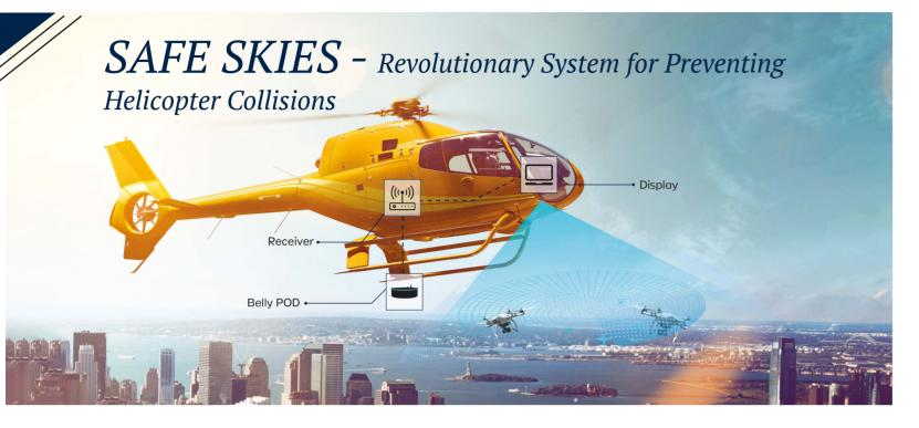
One of the exciting developments at SKYLOCK is "SAFE SKIES," a revolutionary radar-based system for preventing helicopter/drone crashes. Taking into consideration the growing rate of drone incidents such as the recent stoppages at Gatwick and Heathrow airports in the UK along with numerous near-crashes and interferences with first aid and fire-fighting copters, we designed and developed an integrated system that will allow helicopter pilots to avert drone crashes.
